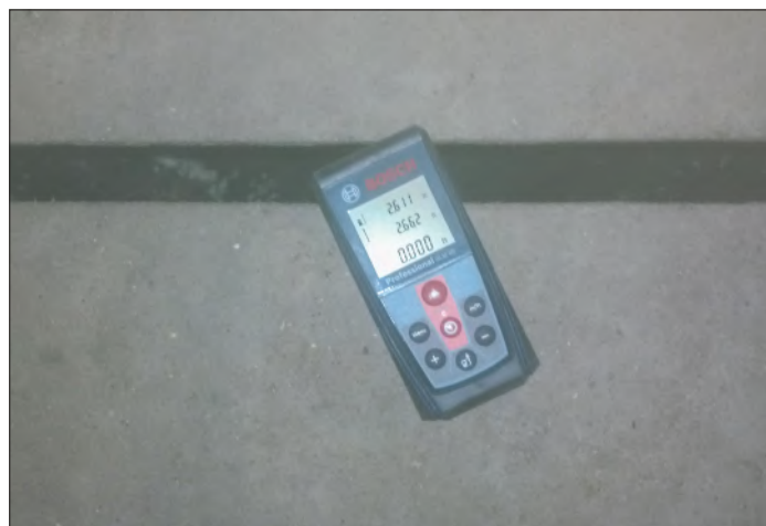
Figure 1. An example of a electronic laser to measure free-board in a hog barn pit.
